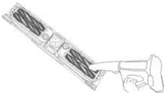
Use a blow dryer to blow away the dust on the surface of the brushes
